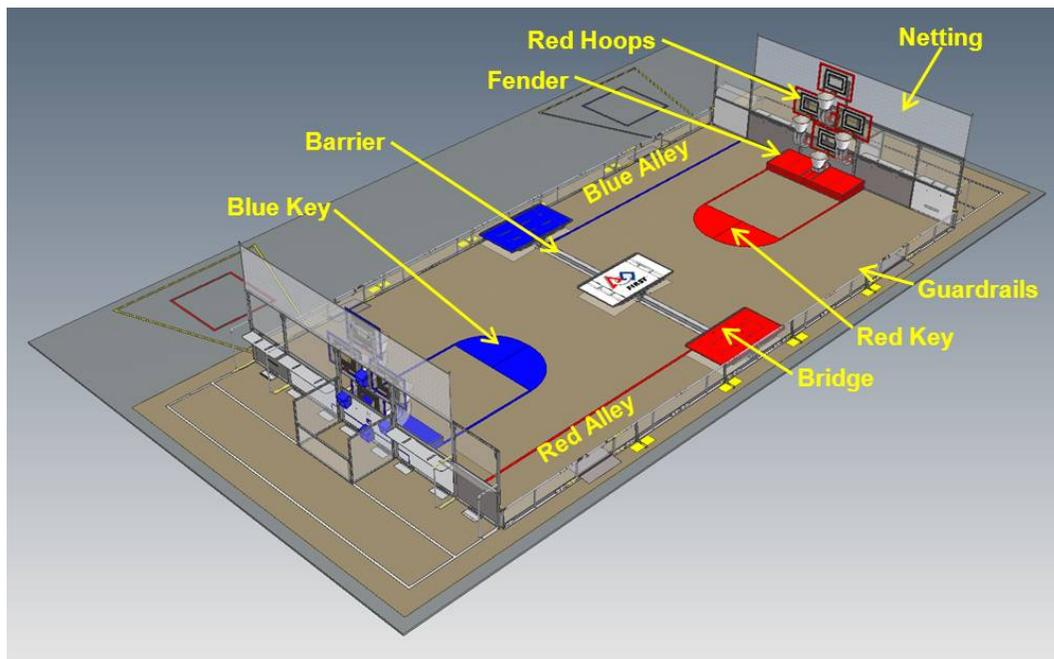
The Alliance Walls are 6 ½ ft high, 27 ft wide, and define the ends of the Court. The Alliance Wall protects the Player Stations, and is composed of a 3 ft high base of diamond plate aluminum topped with a 3 ½ ft high transparent polycarbonate panel.
